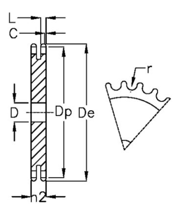
C = 1 D = 20 De = 383.5 Dp = 379.02 For chain size =  $3/8 \times 7/32$ For chain type = 06 B-2 h2 = 5.3
